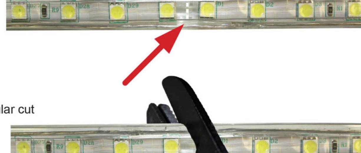
Use a heavy duty shears to make a perpendicular cut between bulbs in the center of the gap.
